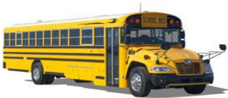
Type C Buses (Conventional) Seating Capacity: 36-83 Fuel Types: Diesel, Propane, CNG, Gasoline, Electric
