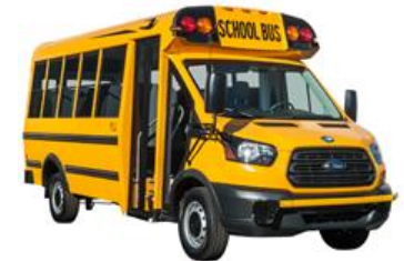
Type A Buses Seating Capacity: 10-30 Fuel Types: Diesel, Propane, Gasoline, Electric (2018)
