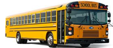
Type D FE Buses (Front Engine, Transit-Style) Seating Capacity: 54-90 Fuel Type: Diesel
