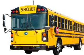
Type D RE Buses (Rear Engine, Transit-Style) Seating Capacity: 66-84 Fuel Types: Diesel, Electric
