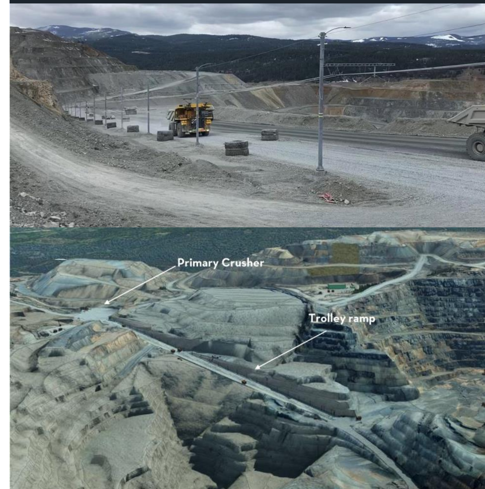
COPPER MOUNTAIN IS THE 1 ST OPEN PIT COPPER MINE IN NORTH AMERICA TO USE TROLLEY ASSIST
