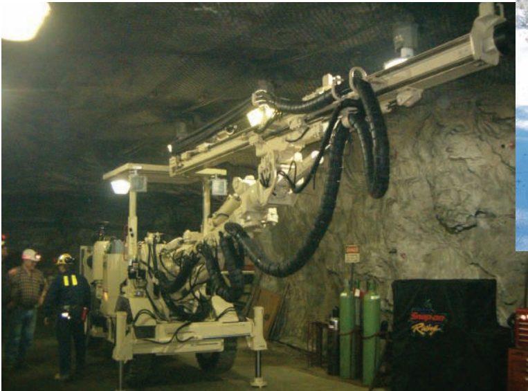
Jumbo drill at Balmat mine
