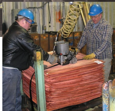
Bill Cook and Robert Harges banding copper cathode at White Pine Copper Refinery
