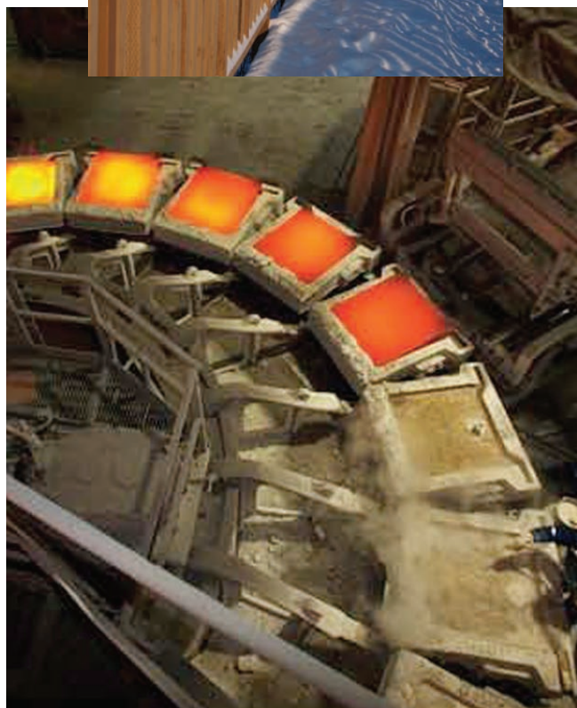
The anode casting wheel in the copper smelter, Flin Flon, Manitoba
