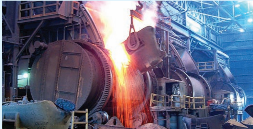
Charging a converter in the copper smelter
