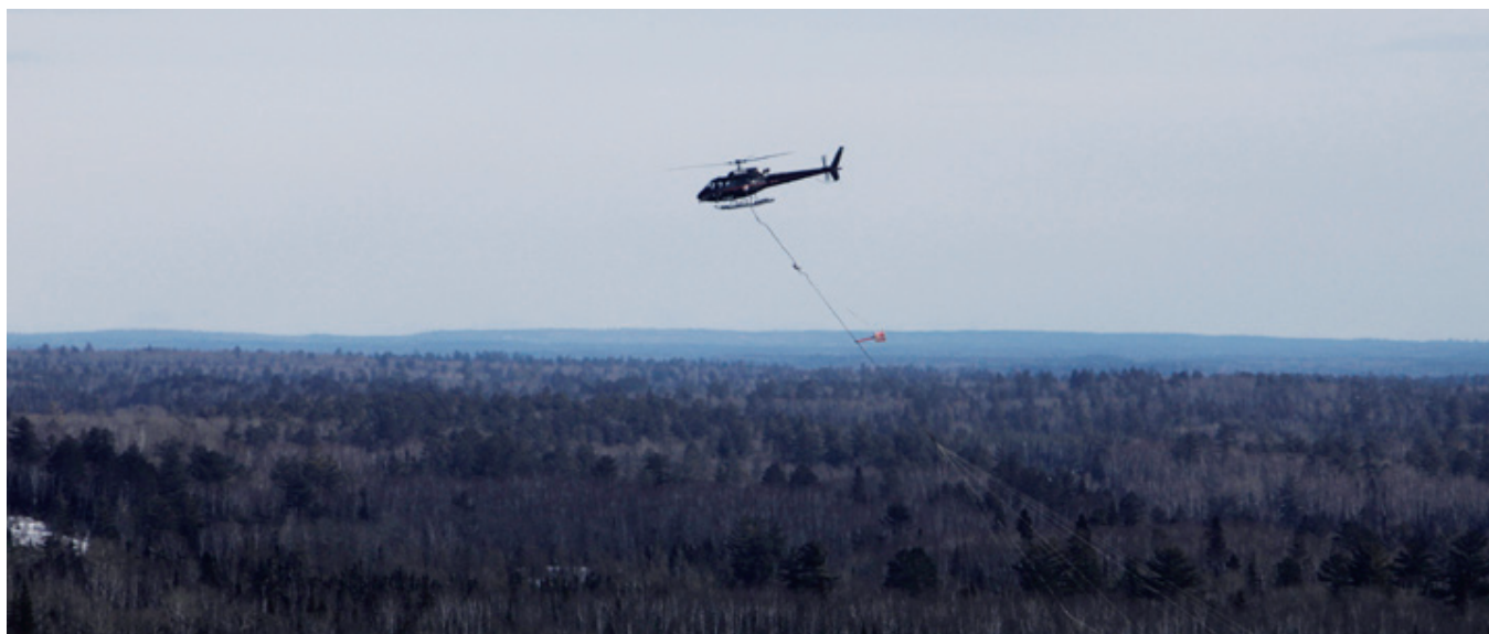
↑ Geophysical surveying conducted at the Back Forty project in northern Michigan. HudBay relies on electromagnetic geophysical technology as one of its primary exploration methods.
