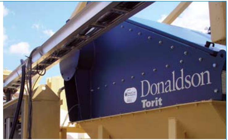
Torit® PowerCore® installed on a mobile concrete mixing plant
