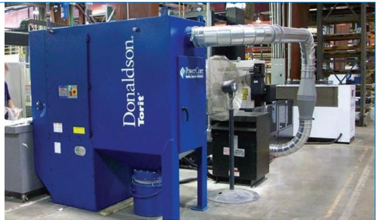
A Torit PowerCore system used to collect metalworking fumes in a laser cutting operation
