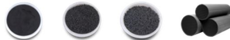
Powdered activated carbon Granular activated carbon Pelletized activated carbon Activated carbon honeycombs
