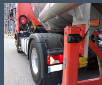
Proximity protection technology alerts drivers to the presence of pedestrians. Different types of technology are being implemented at Dow sites around the world.
